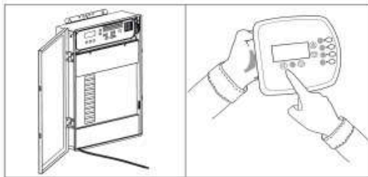
1. Disable priming on automation control system.
