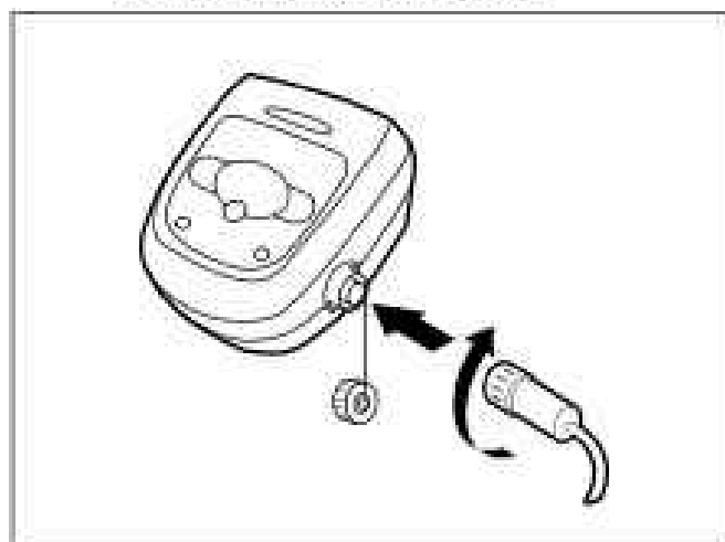
Figure 11. Connecter un câble flottant
