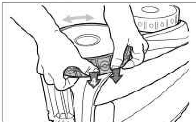
Figure 36. Push the Tire Into Place on the Wheel
