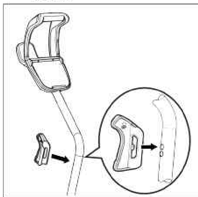
Figure 7. Snap Cleaner Hook into Place
