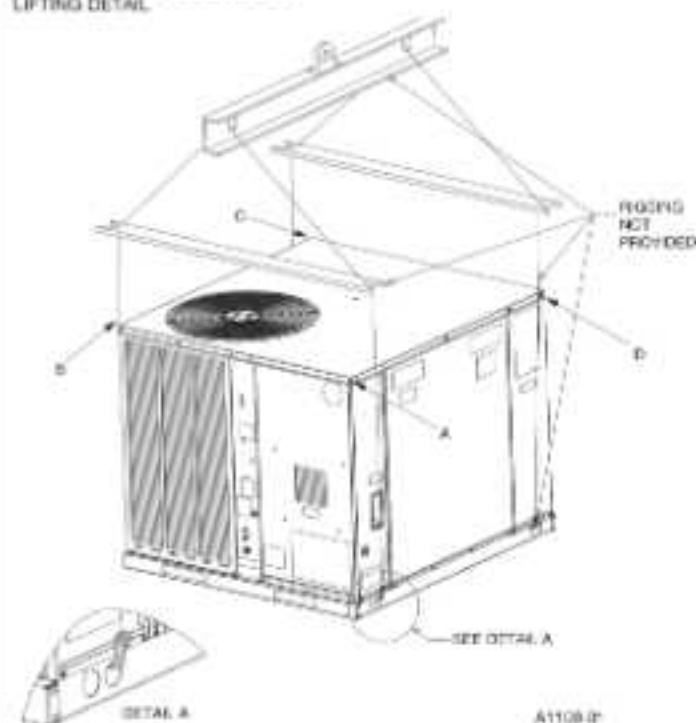
FIGURE 6 PACKAGED AIR CONDITIONER LIFTING DETAIL
