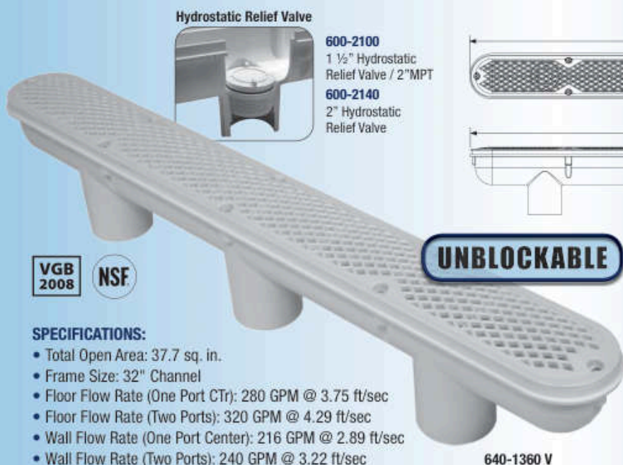
Hydrostatic Relief Valve
