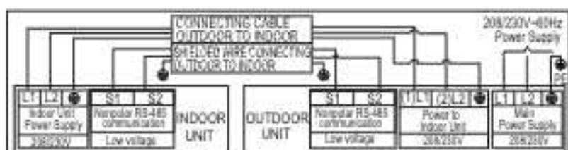
Connection Diagram (36K/48K/60K)
