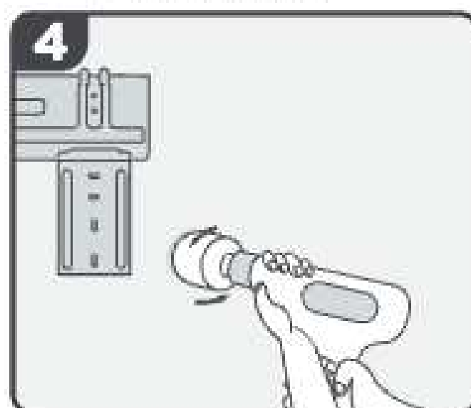
Drill Wall Hole
